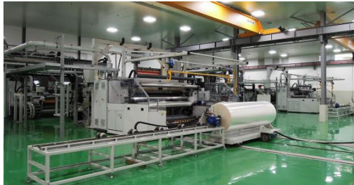
New CPP production line in Melaka
